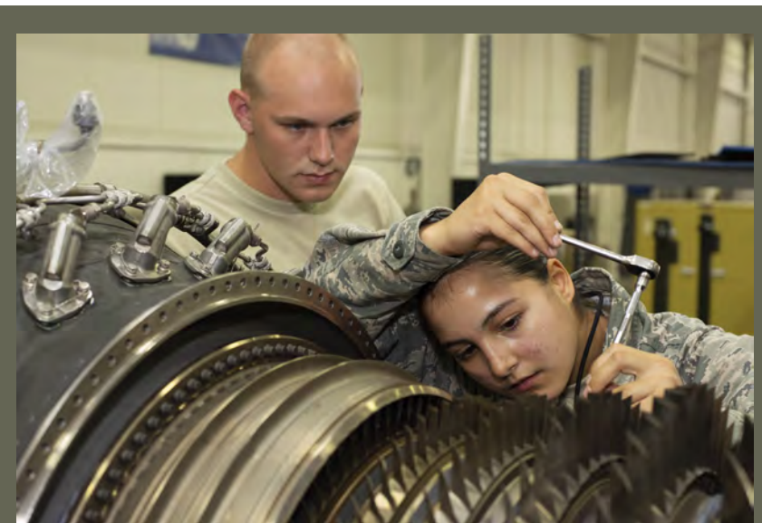
Airman 1st Class Mariana Salazar, an aerospace propulsion Airman assigned to the 509th Maintenance Squadron jet propulsion flight, trains to perform maintenance on an F-118 engine on July 9, 2019, at Whiteman Air Force Base, Missouri. Salazar and other members of his flight run diagnostic tests and perform regular maintenance on F-118 engines on a daily basis to ensure the readiness of the B-2 Spirit fleet at Whiteman AFB. The jet propulsion flight achieved the highest readiness rate across the active-duty Air Force. (U.S. Air Force photo by Staff Sgt. Kayla White)
