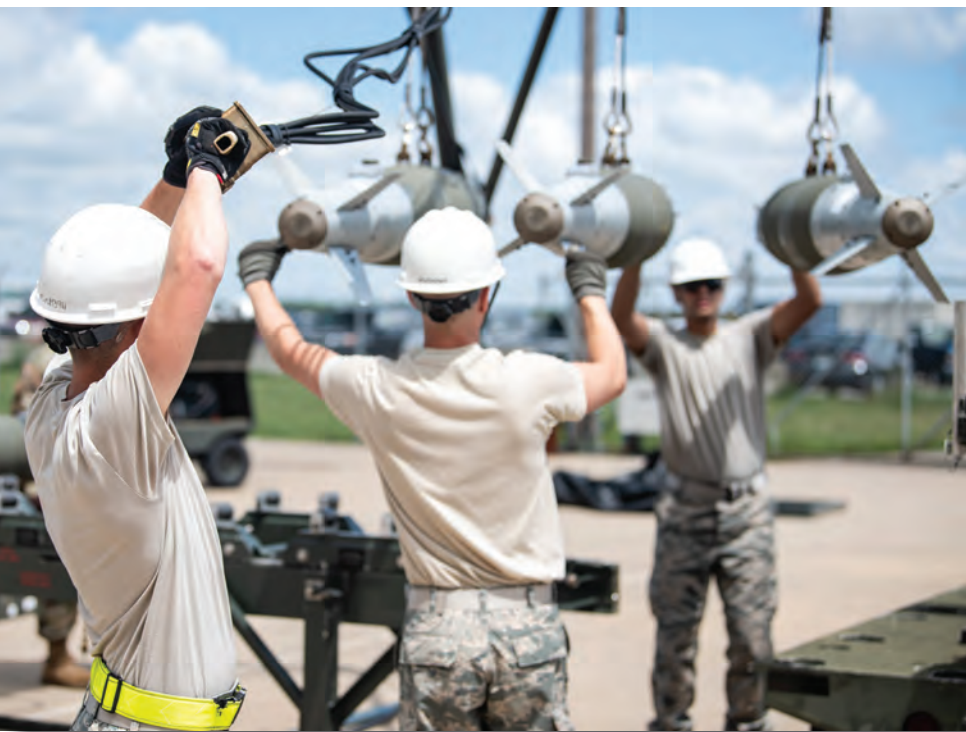
Airmen from the 509th Munitions Squadron raise munitions onto the Munitions Assembly Conveyor (MAC) during the Global Strike Challenge (GSC) at Whiteman Air Force Base, Missouri, June 24, 2019. The MAC is designed to provide a mobile capability to rapidly assemble and disassemble conventional munitions and provide a means to load and unload to and from a munitions handling trailer or vehicle. (U.S. Air Force photo by Senior Airman Thomas M. Barley)
